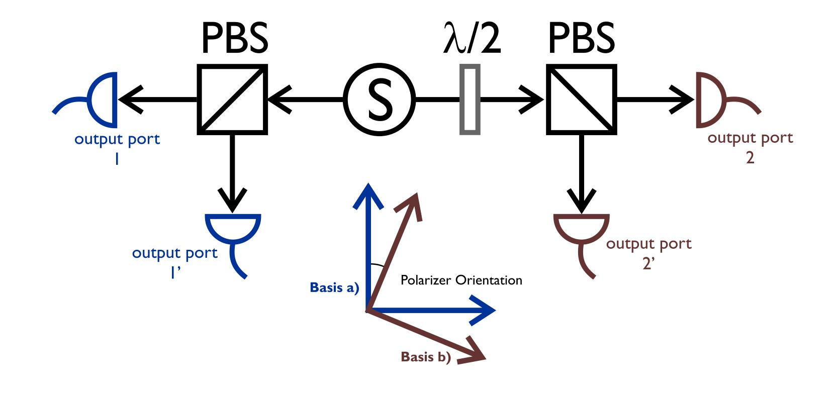
S: source of entangled photons λ/2 plate: rotates the polarization by an angle PBS: polarizing beam splitter, measures the polarization state
